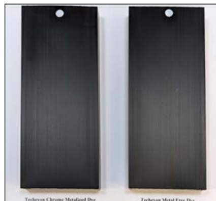
Figure 4. Anodized samples, showing a black dye with metal (left) compared to a black dye without metal (right). The metal-free sample exhibits a minimal color difference, with a delta E value of just 0.745, when compared to standard chrome metallized black dye. (Photo: © Techevon.)
