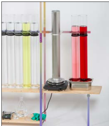
Figure 3. Anodizing chemical testing of yellow, pink, and red coloring baths made from plant-based dyes. (Photo: © Loop Loop.)
